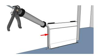
To install the next piece next to the end piece, internal or external corner, a continuous vertical line of glue must be applied to the side. Stay about 2 cm away from the edge when doing this.
