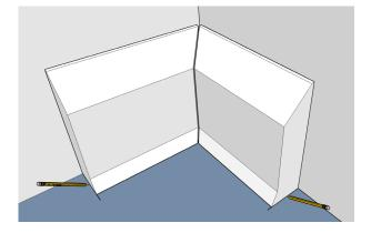
For inside corners and outside corners, it is best to put the pieces in place first (without glue!) and mark the ends on the floor.
