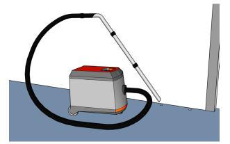
Make all holes 100% dust-free and clean. The holes must be dry to achieve good adhesion!
