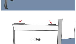
Before installing the end pieces, the door frames must be in place or clearly marked.
