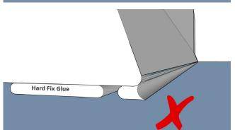
For the bottom joint, the tape is positioned on the kerb just above the rounding. On the floor, the tape can be positioned in line with the footing or slightly in front of it.
