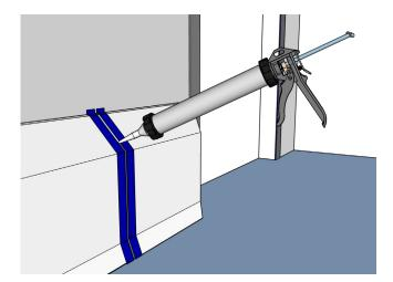
Fill the vertical joints between the kerbs completely with a little extra that comes out of the joint.
