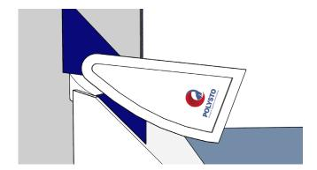
Repeat the steps described in finishing the vertical joint. For smoothing, use the rounded side of the tool as shown.
